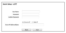
Select **Static IP** if the IP Address/ Subnet Mask/ Gateway and DNS server address have been provided by your ISP. Then please enter server IP address or domain name provided by your ISP, and also enter the corresponding parameters.
