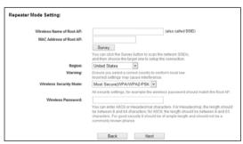
b. Click Survey button on the Wireless Repeater page, and then AP List page will appear. Find the SSID of the Access Point you want to access, and click Connect in the corresponding row. For example, the second item is selected. The target network's SSID will be automatically filled into the corresponding box.
