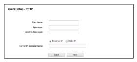
Select **Static IP** if the IP Address/ Subnet Mask/ Gateway and DNS server address have been provided by your ISP. Then please enter server IP address or domain name provided by your ISP, and also enter the corresponding parameters.
